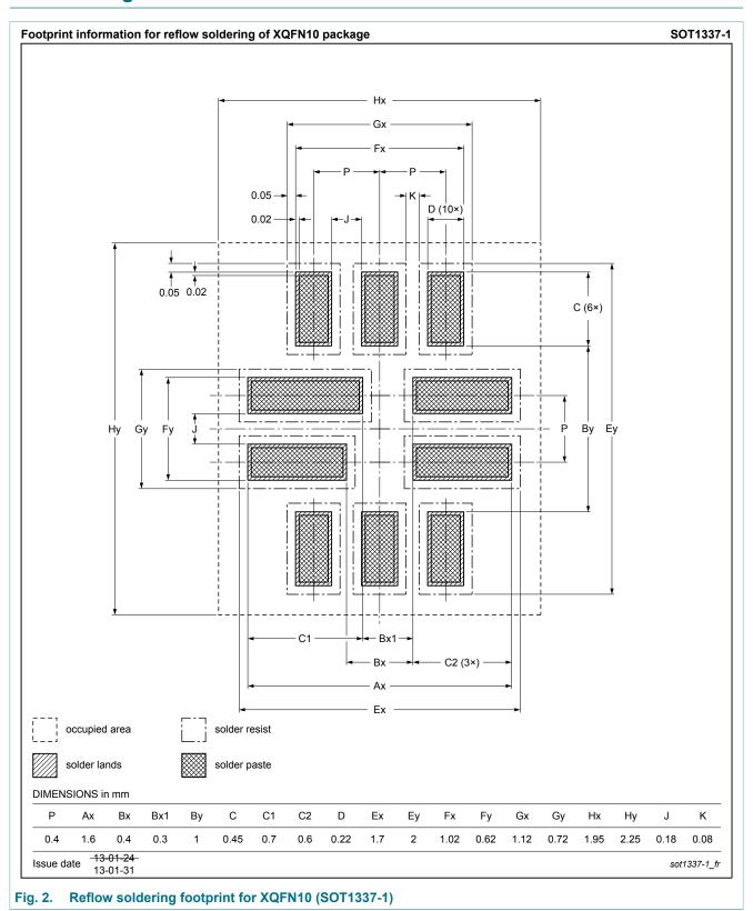
plastic, extremely thin small outline package; 10 terminals; 0.4 mm pitch; 1.3 mm x 1.6 mm x 0.5 mm body
