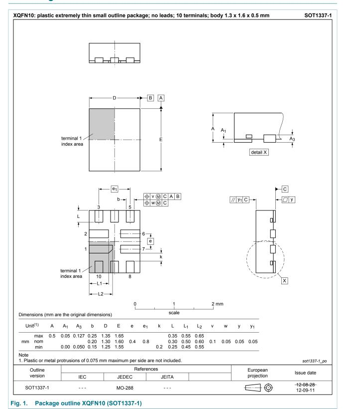
plastic, extremely thin small outline package; 10 terminals; 0.4 mm pitch; 1.3 mm x 1.6 mm x 0.5 mm body
